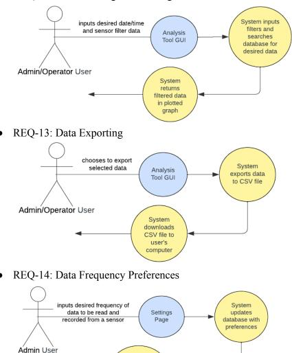
System reads and records data from sensor at new frequency
